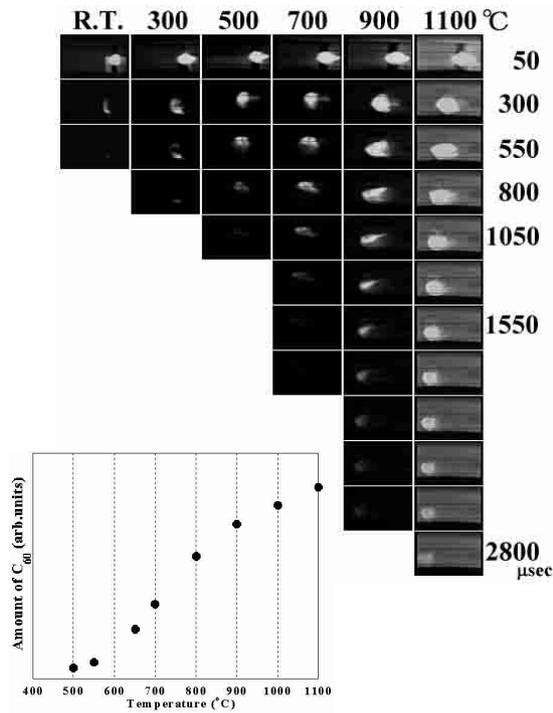
**Fig. 1.** Time and spatial evolution of emission by the plume of carbon nanoparticles immediately after laser irradiation of a graphite rod (each image covers an area of 28 mm × 16 mm).
