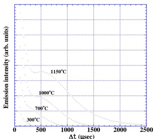
**Fig. 5.** Change in the emission intensity of carbon nanoparticles obtained with a bandpass filter at 694.3 nm. Each set of data was obtained at different ambient temperature (1150 °C, 1000 °C, 700 °C, and 300 °C, respectively).
