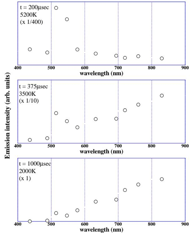
**Fig. 2.** Typical emission profiles of carbon nanoparticles ejected from the surface of graphite rod at  $\Delta t = 200 \mu\text{s}$ , 375  $\mu\text{s}$ , and 1 ms, respectively. The ambient gas temperature is kept at 1150 °C.
